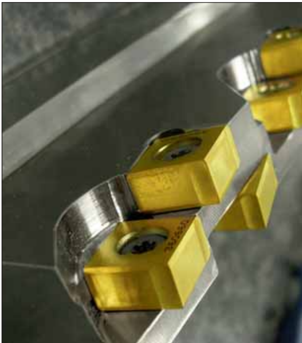
PULL-BROACHING is the fastest way to produce slots in turbine discs and with our solutions using indexable carbide inserts the cutting speed can be increased four fold; productivity will be doubled and no more tooling regrinding operations will be required.
