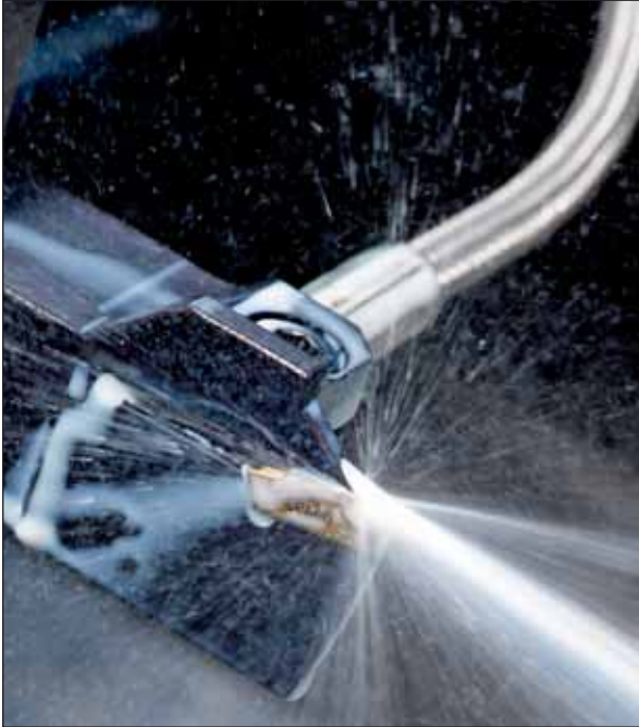
JETSTREAM TOOLING enables high velocity coolant to be delivered close to the cutting edge eliminating chip evacuation issues in a wide range of difficult to machine materials.
