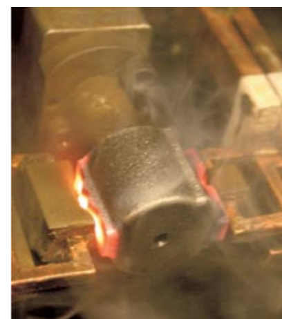
▲ Induction hardening is carried out on the production line.
