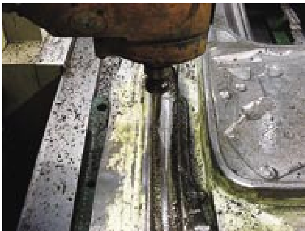
One of the simulations conducted at the 2003 Open Day with our Minimaster completing a 3D run on a mould for the MPV Sharan in the machinery section (Toolshop department).
