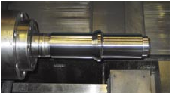
The rough machining operation has been completed.
