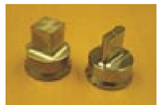
The punches for Kingsland machines are usually produced using 50 mm diameter Seco R220.99 milling cutters. The inserts are SONX 12 of grades T20M and T25M. The cutting speed is 190 m/min.
