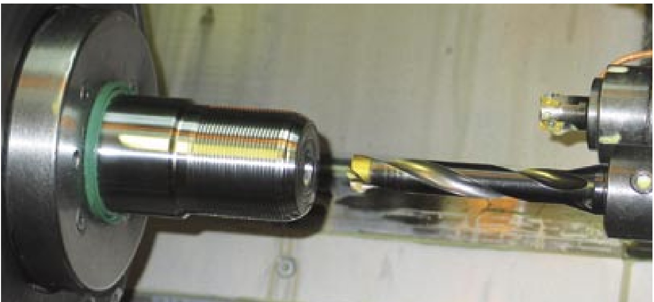
CrownLoc can drill 300 of these holes before the crown needs changing.
