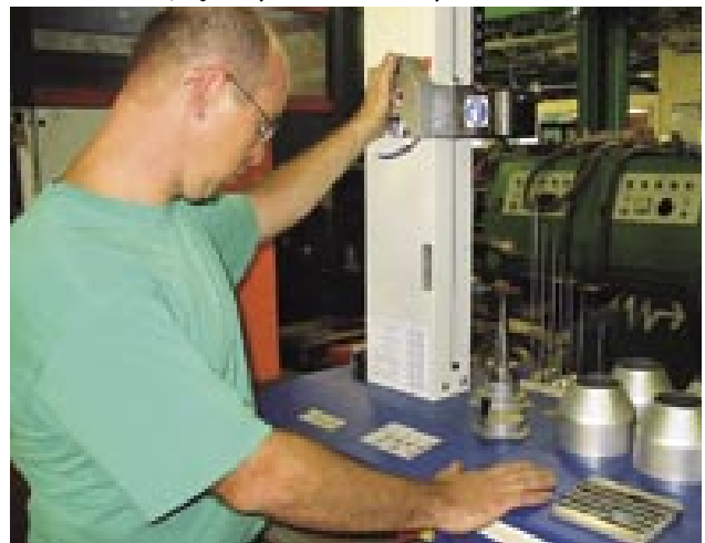
Shrink fit operation in an EPB machine with Jabro cutters
