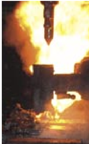
Drop forging in progress.
