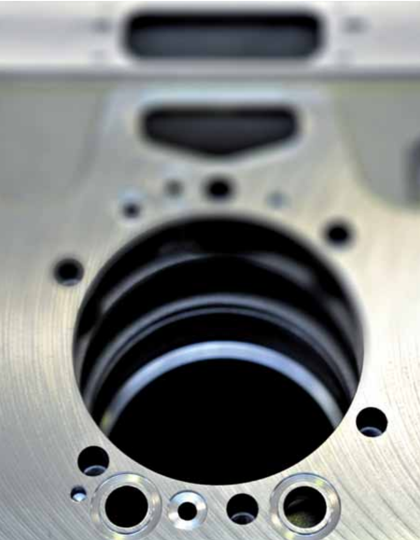
The Minimaster Plus works on 90 engine blocks before requiring a tool change.
