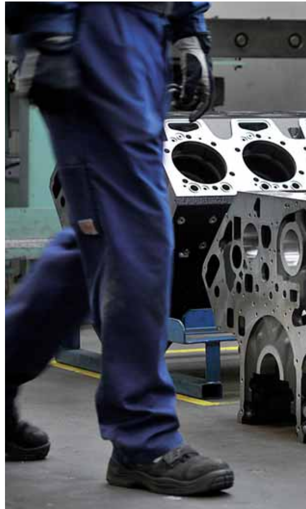
The Minimaster Plus works on 90 engine blocks before requiring a tool change.
